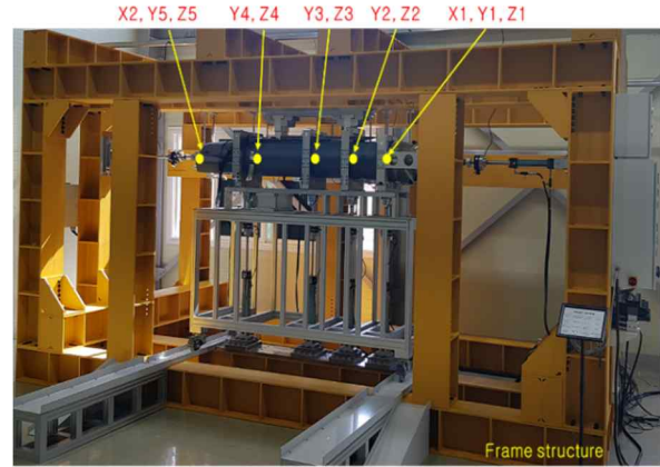
Fig. 9 Full-Scale Static Test for Sensor Pod
