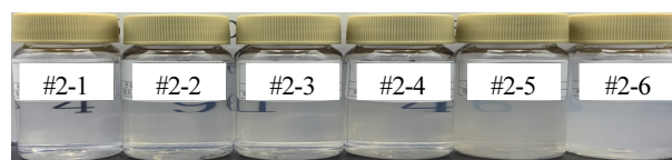
Figure 3. Results of composition experiment for turbidity test according to different polyols in Table 4.
