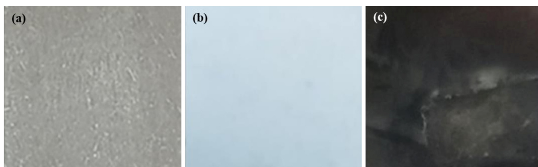
Fig. 5. Photographs of the anode before (a), and after (b) one hour's reaction at 0.18 V and 50°C. The silver anode was initially gray (a) but became white (b) due to the oxidative deposition of AgCl on its surface. For comparison, the photograph of the anode after the same reaction at 0.3 V and 50°C is shown in (c). Here, the anode turned black due to the formation of black \text{Ag}_2\text{O} particles.
