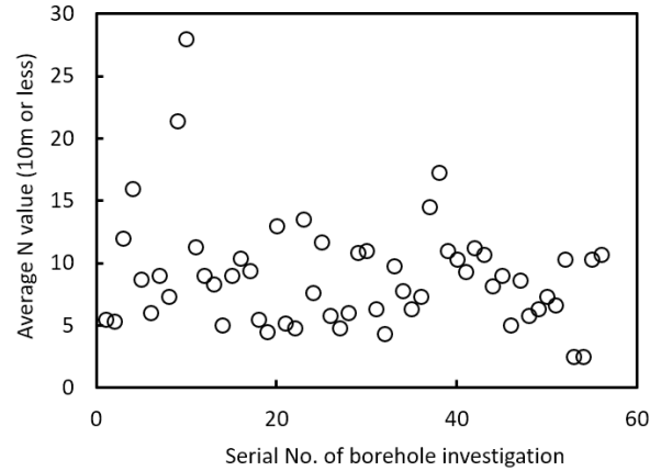
Fig. 4. Average SPT N values from crest to a depth of 10m (results of 56 boreholes in 29 reservoirs)
