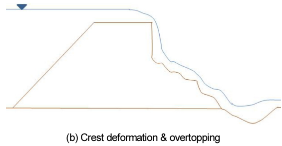
Fig. 1. Main potential failure modes of embankment by earthquake loads [1, 4]
