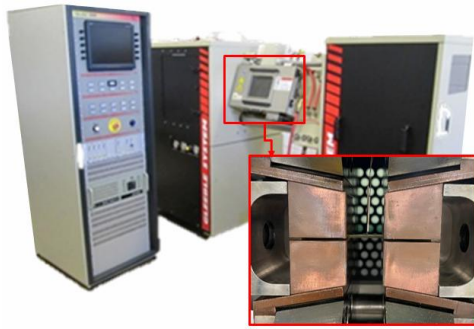
Fig. 3 Gleeble 3500 System for testing the oxide layer thickness of un-coated boron steel sheet
