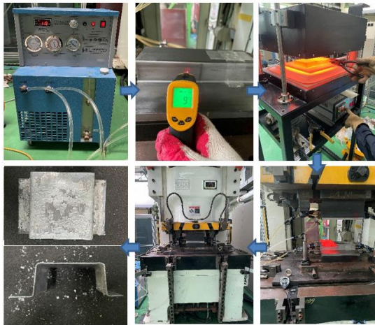
Fig. 1 Hat-type hot stamping test with un-coated boron steel sheet
