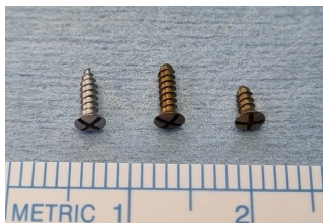
Fig. 3. Types of screw tips used in internal fixation of facial bone fracture surgery. Notice the length of the screw and the shape of the tip. The long screws (left and middle) are 6 mm, and the short screw (right) is 4 mm. The blunt and short screw (right) was used in complex orbital fracture patients to prevent balloon rupture.
