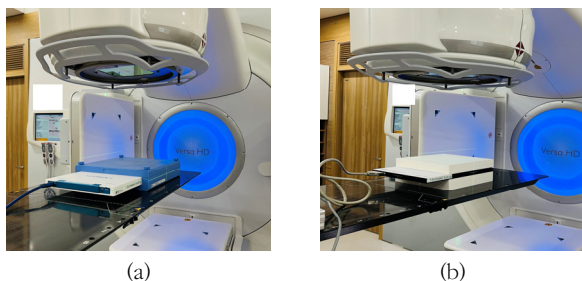
Fig. 1. Experimental setup for delivery quality assurance (DQA) using (a) MapCHECK™ and (b) OCTAVIUS™.
