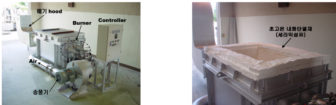
Fig. 4. Installing test bodies in furnaces
