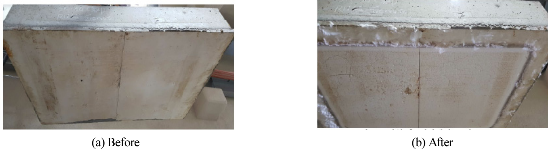
Fig. 6. Changes before and after fire resistance test
