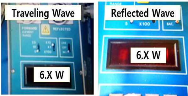
Fig. 8 Traveling and Reflected Waves of RF Cable
