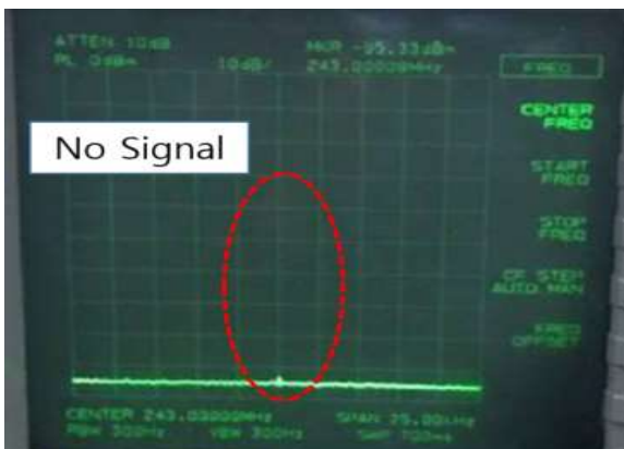
Fig. 19 Measurement Result of Commercial Broadcasting Reception Signal(No Signal)
