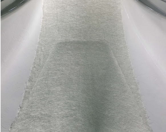
Fig. 10 Lamination of GFRP on the Mold
