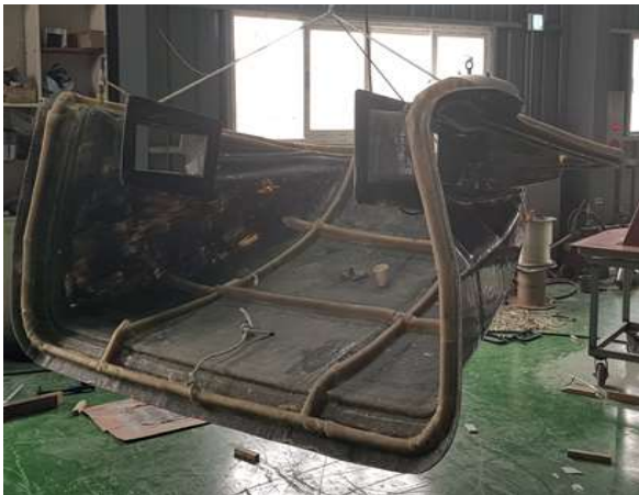
Fig. 11 Demolding of Prototype to the Mold
