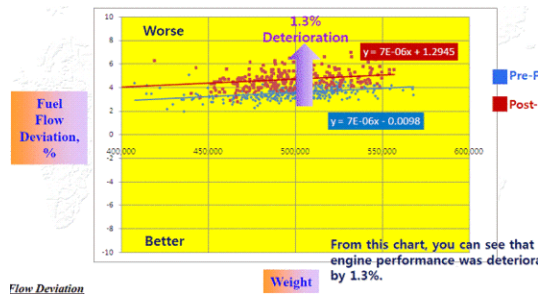
Fig. 12. Changes in engine performance after installing the performance enhancement package
