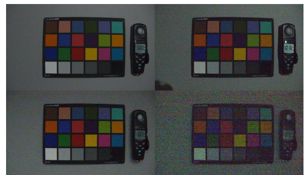
Fig. 8. Raw colorchecker image visualized by ISP (50lux, 10lux, 1lux, 0.1lux from left top to right bottom)
