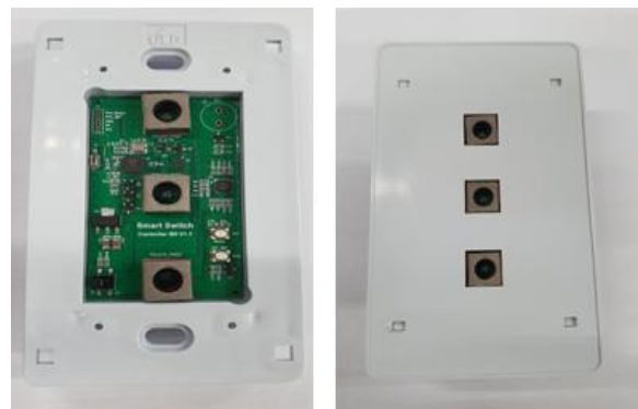
Fig. 14. Smart Wall Switch with IEEE 802.11b/g/n
