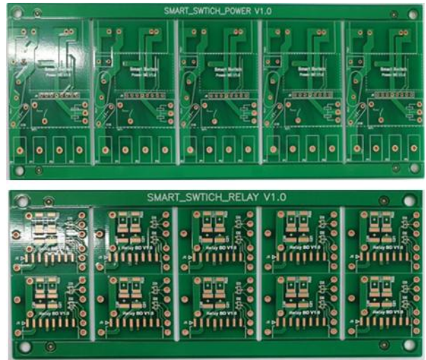
Fig. 6. Power Board(Top) and Relay Board(Bottom) Sample
