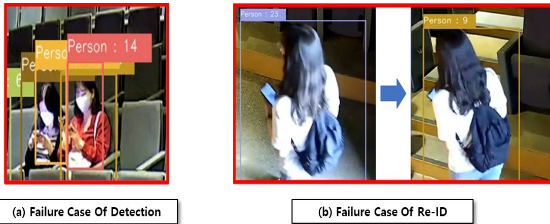
Figure 7. Failure Case of Detection & Re-ID (a) Failure Case of Detection, (b) Failure Case of Re-ID
