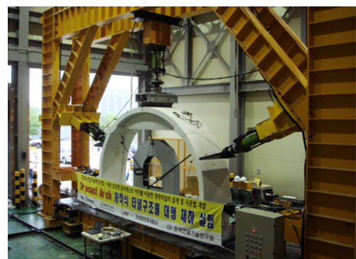
(a) The rib-reinforced precast arch structure on the assembly
