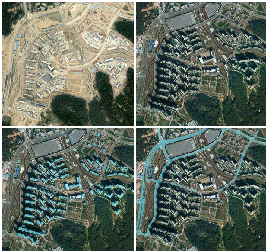
<Figure 4> Analysis of Land Cover Changes Using DeepLab V3. (Top left: Image of 2018. Top right: Image of 2020. Bottom left Detected changes in buildings. Bottom right: Detected changes in roads)
