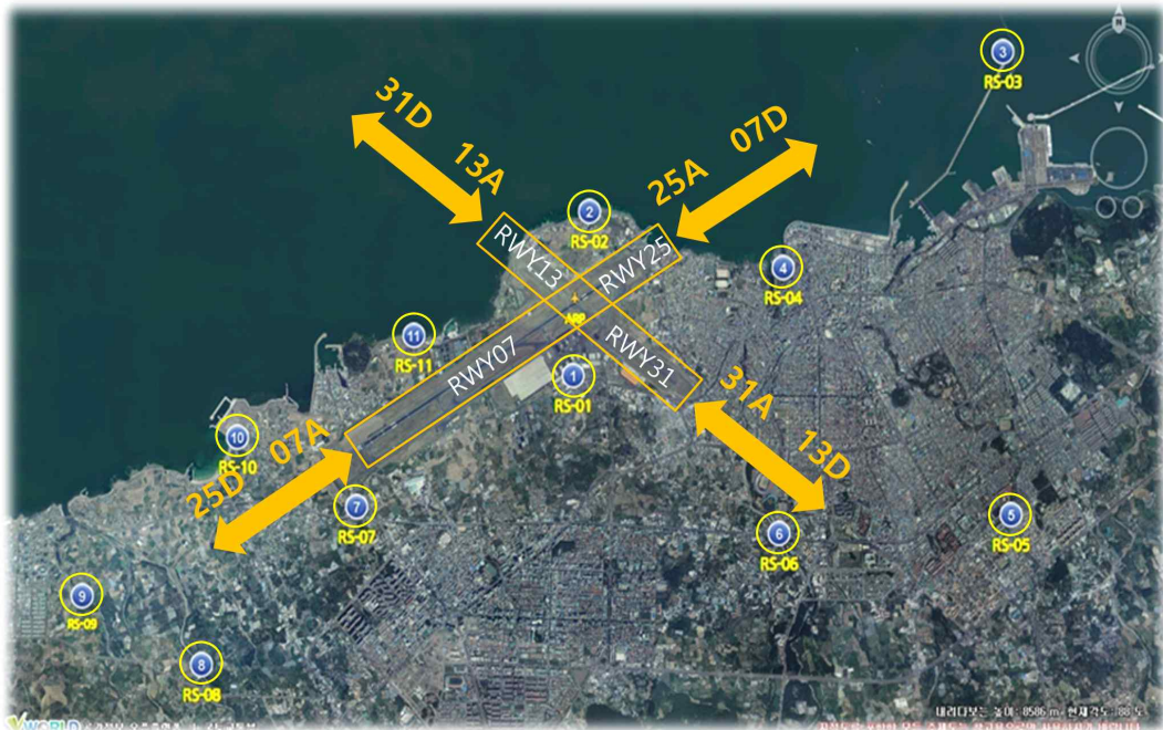
Fig. 1. Location of 11 LLWAS sensors and runway corridors at Jeju International Airport
