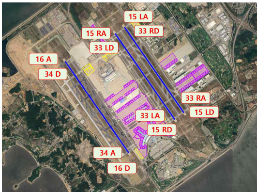
Fig. 4. Runway characteristics of RKS1 input to KMAP-LLWS. The figure panel is derived from AIM (aim.koca.go.kr)
