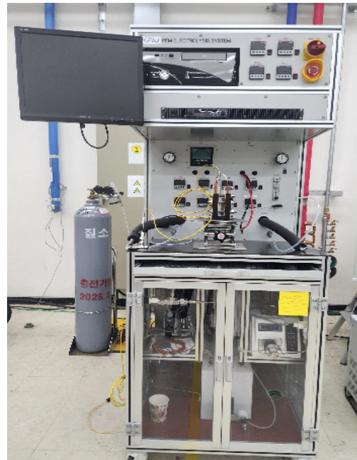
Fig. 3. Stack performance test station
