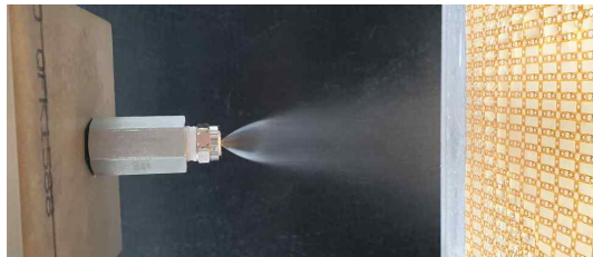
Fig. 8. Spray impingement on a vertical plane wall
