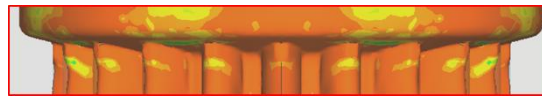
(c) Underfill occurrence in the taper shape die of 2nd cold forging
