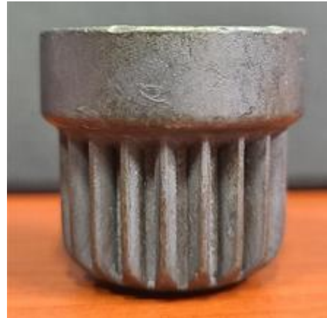
Fig. 19 1st cold forging product of Spur Gear
