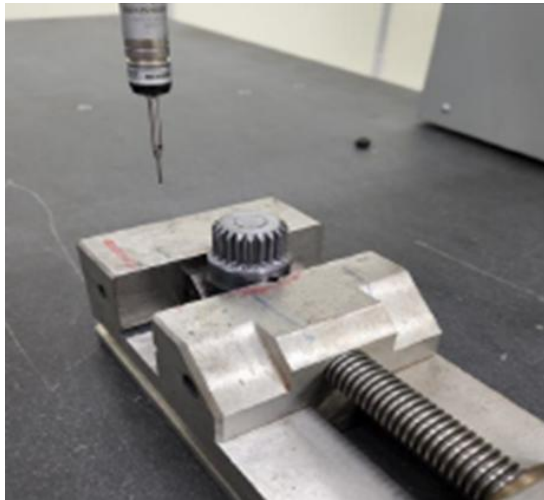
Fig. 21 Outside diameter measurement of Spur Gear product
