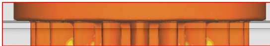
(c) No underfill in the square shape die of 2 nd cold forging
