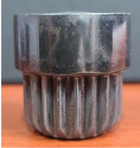
Fig. 20 Final cold forging product of Spur Gear
