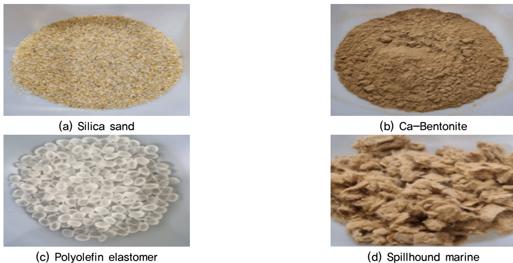
Fig. 1. Materials for selectively block barrier
