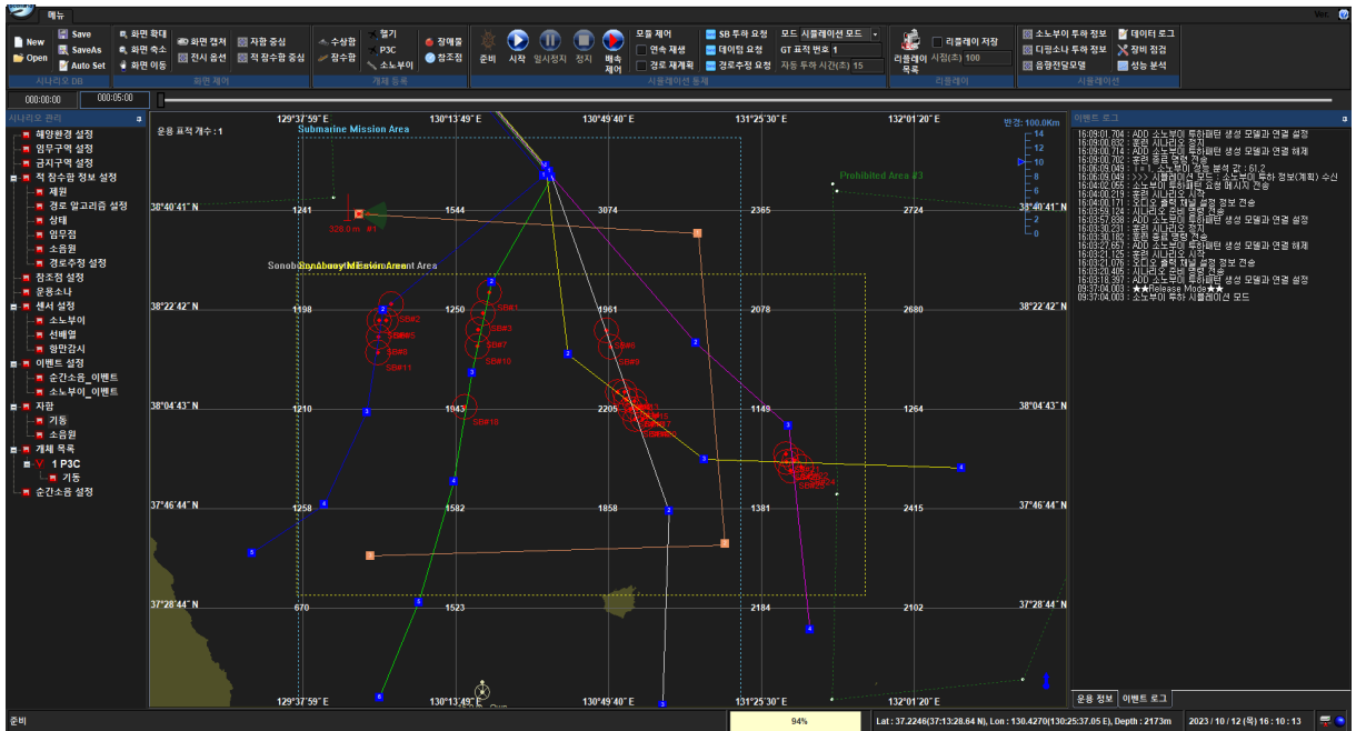
Fig. 24. Sonobuoy deployment according to optimization
