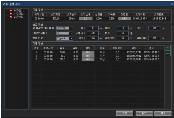
Fig. 15. Route of surface ship and submarine, submarine size, recognition setting in mission area
