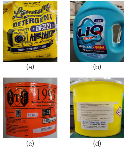
Fig. 2. Types of detergents used in laundry tests: (a) commercial detergent(powder), (b) commercial detergent(liquid), (c) standard detergent 1, (d) standard detergent 2
