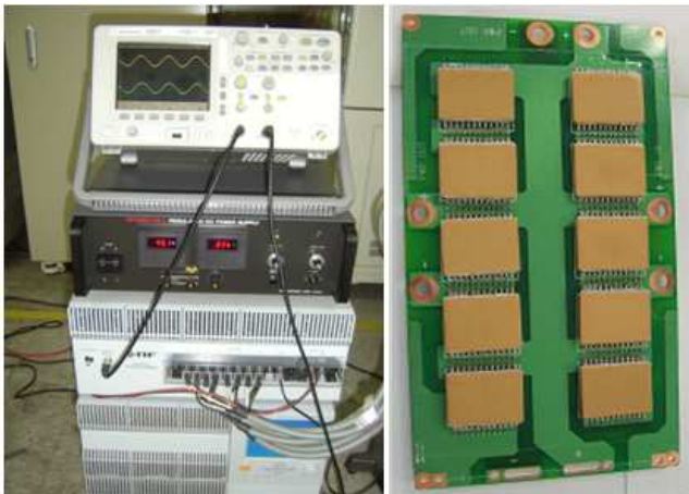
Fig. 1. Photos of a ripple current test system (left) and a capacitor module (right).
