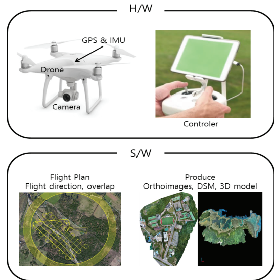
Fig. 1 Configuration of UAV-Photogrammetry system
